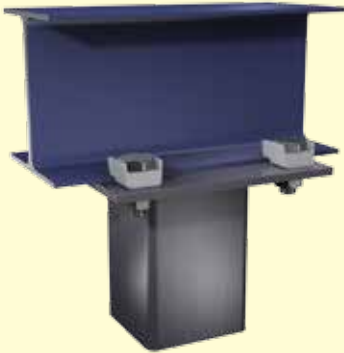
Column end plate to I-Section
