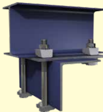
Angle section below an I-Section at 90 degrees
