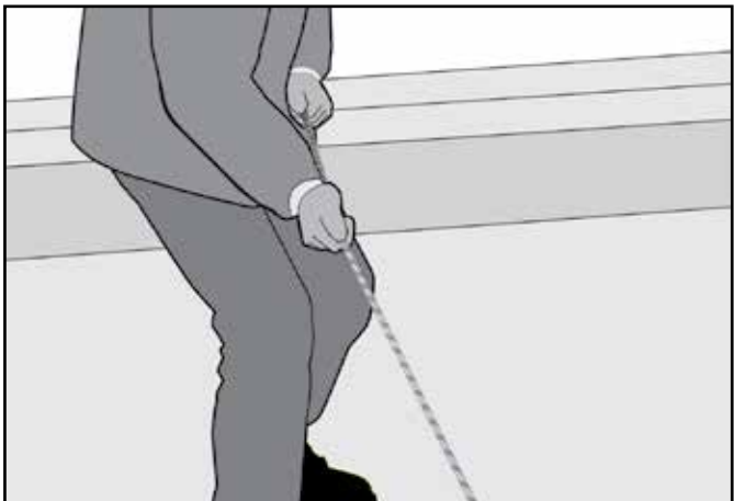
c. Start walking towards the area where the casualty has fallen whilst still holding the Rescue Rope Grab. When you reach this area, kneel down and continue to pull out sufficient rope to reach the "D" ring on the casualty's harness.
