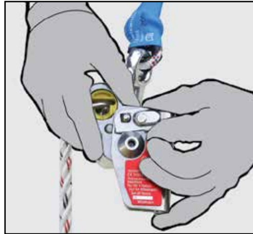
f. Turn the Rescue Rope Grab over and push the lever in an upwards direction.
